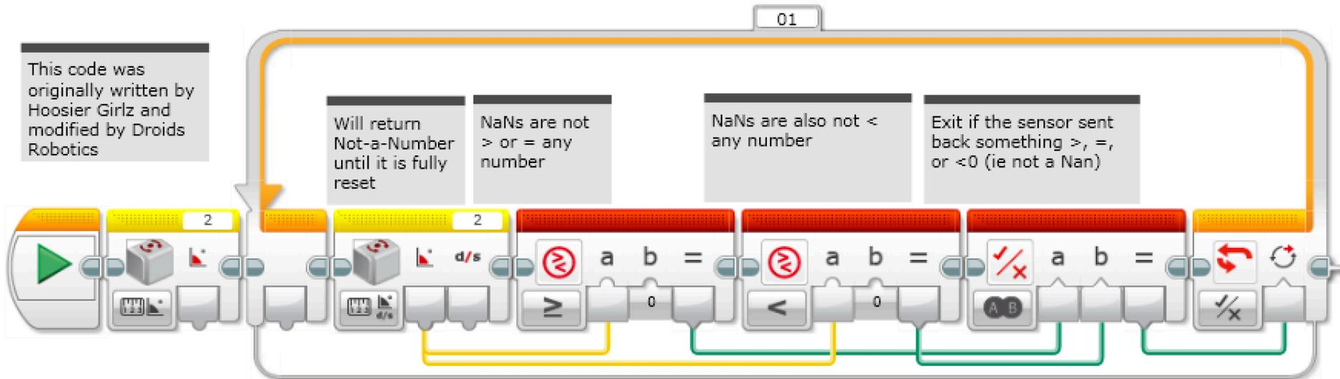
This version of the calibration leaves the gyro in rate+angle mode. This is useful if you use the rate output.
