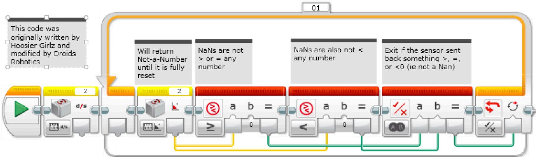
This version of the calibration leaves the gyro in angle mode. This is probably the most common way to use the gyro. This code takes about 0.1sec to run.
