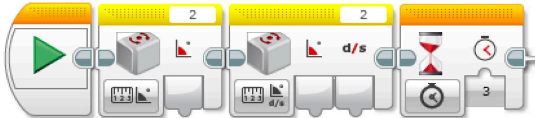
By reading the angle of the gyro then the rate+angle the gyro sensor gets recalibrated. Make sure to run these blocks when the robot is still.
