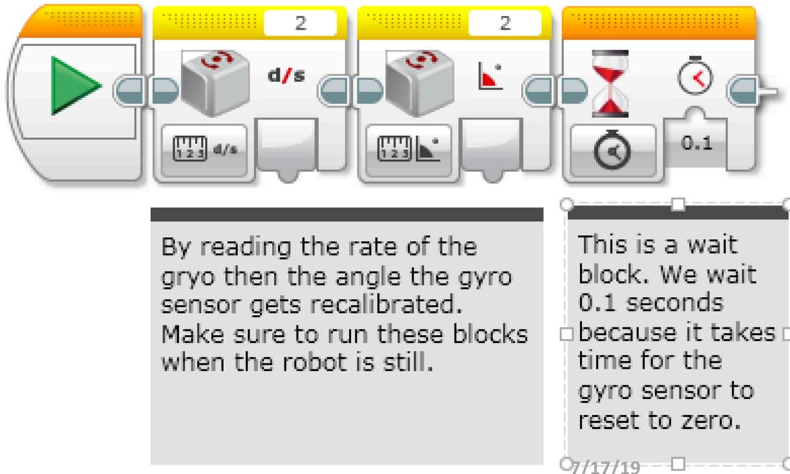
Note that in the rest of your program, you should only use the “angle” modes of the gyro. Using the “rate” or “rate and angle” mode will cause the gyro to recalibrate.
