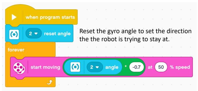
Start moving and adjust the steering based on how far off the robot is from its target
