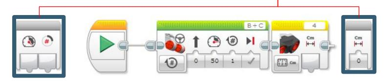
B. Wire up the My Block by dragging a data wire from each parameter to its corresponding slot on the move steering block and sensor block.
