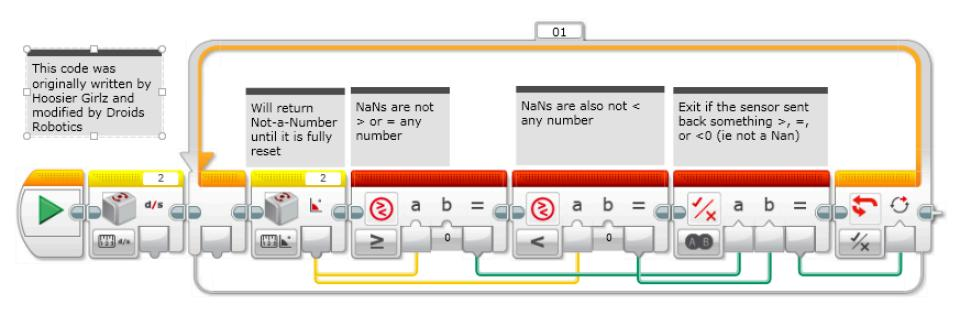
This version of the calibration leaves the gyro in angle mode. This is probably the most common way to use the gyro. This code takes about 0.1sec to run.
