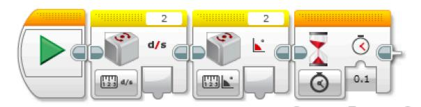
By reading the rate of the gryo then the angle the gyro sensor gets recalibrated. Make sure to run these blocks when the robot is still. This is a wait block. We wait 0.1 seconds because it takes time for the gyro sensor to reset to zero.
