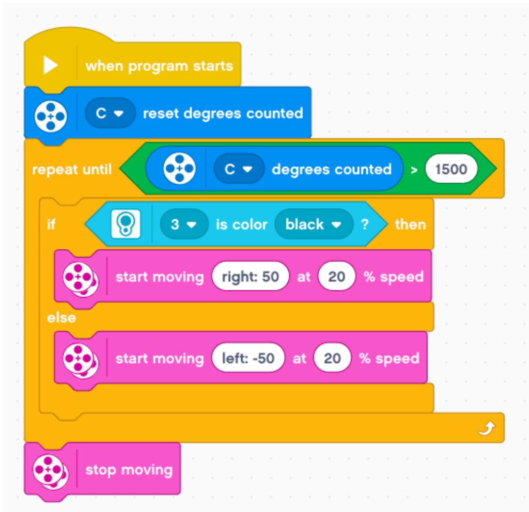
Reset rotation sensor (Reset Degrees Counted) on Motor C
