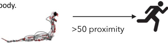
If the robot is less than 50 proximity away, it will attack (open its mouth), back off and turn.
