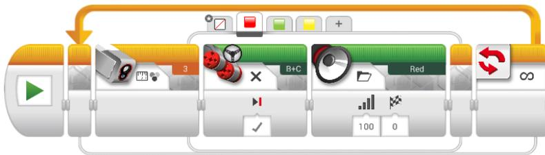
When the robot reads red, the motors stop
