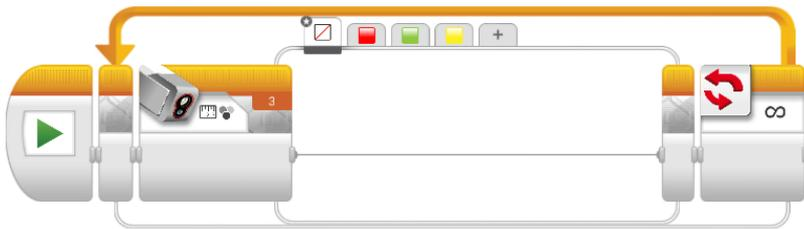
When the robot reads no color the robot does nothing
