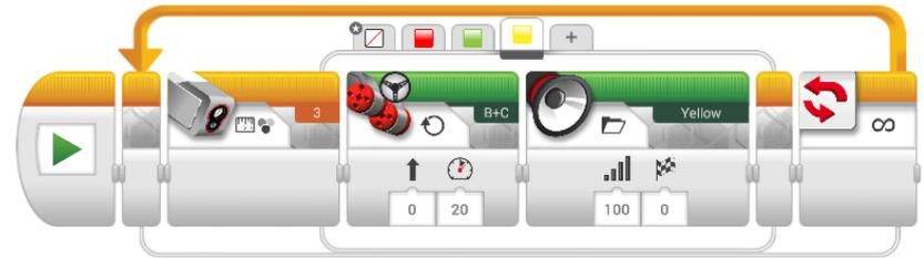
When the robot reads yellow, the robot moves at 20 power
