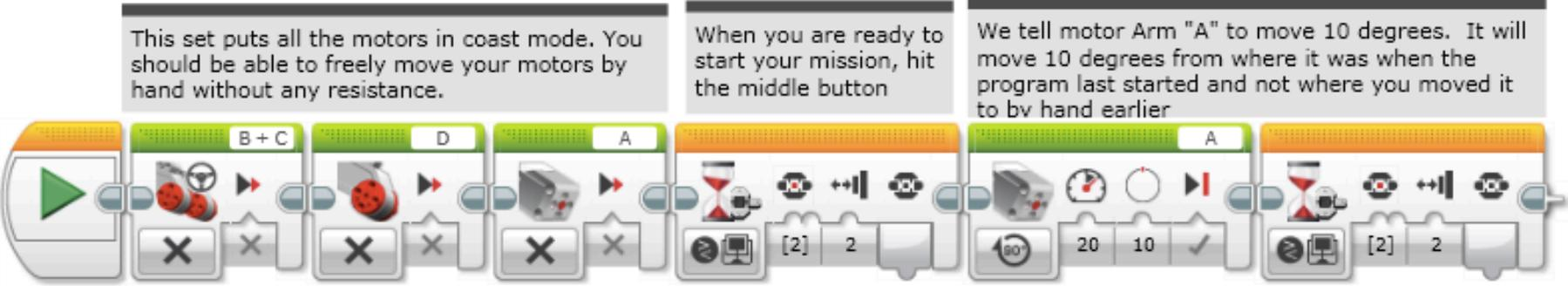
This code shows that the motor arm (A) will not be predictable no matter how much you reset the arm by hand. It's movement is based on where the arm last was. Move the arm by hand at least 90 degrees to see the difference.
